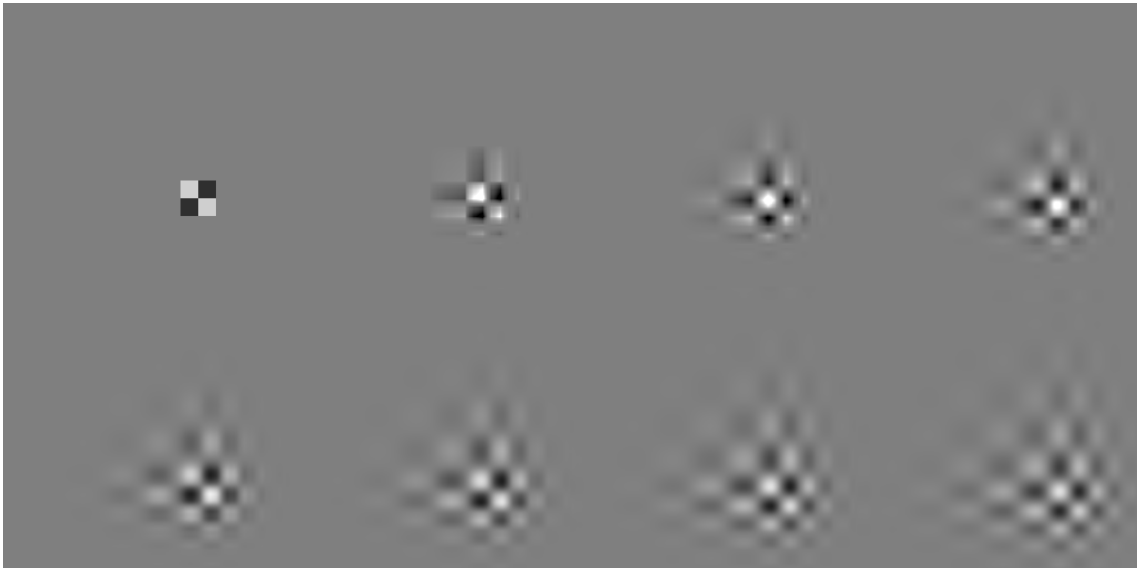
Figure 3.4: A typical 2D-Daubechies wavelet on the diagonal (at position 14-14 in the dyadic decomposition), where the number of vanishing moments goes from p = 1 (top left) to p = 8 (bottom right).
