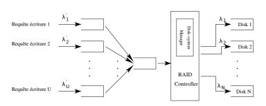
Fig. 1. Requests flow in a RAID storage system
