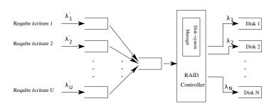
Fig. 1. Requests flow in a RAID storage system
