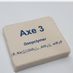
Polycondensation reaction from silicate solution clay
