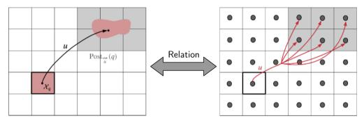
Additional non-determinism resulting from the discretization The number of cells grows exponentially with the dimension of the state space
