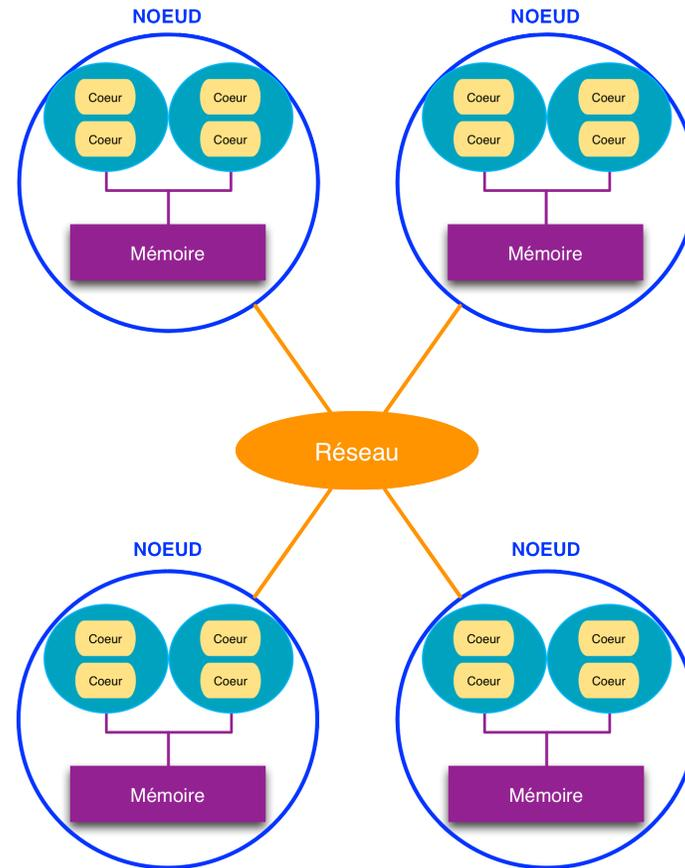
4 nodes (2 processors/2 cores) with hybrid memory
