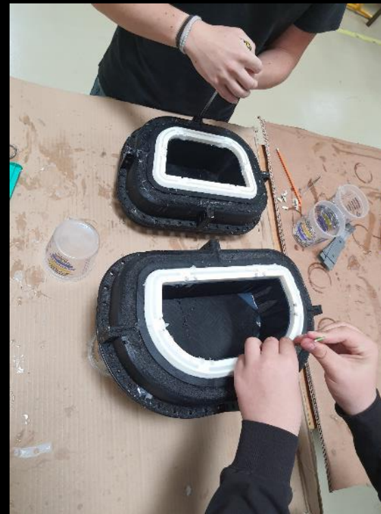
Molding of the silicones skins, P. Roux, M. Guirault (Femto-ST/S.MART)
