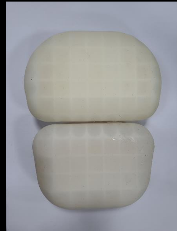
Molding of the silicones skins, P. Roux, M. Guirault (Femto-ST/S.MART)
